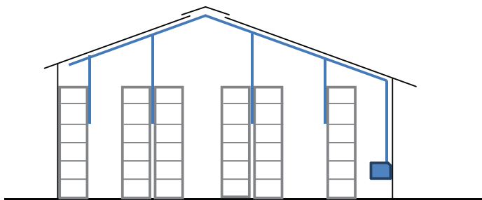
Figure 19. Example of drop-down pipes for in-rack ASD
